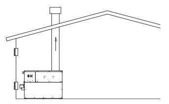
Figure 7 – Outside Combustion Air - Two Openings
